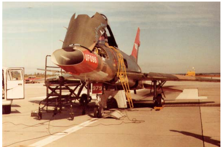
Technicians swarm over the “City of Terre Haute” QF-100 being readied for takeoff on the runway at Tyndall AFB. Note the MCU 800 feet behind the drone on the runway centerline.
