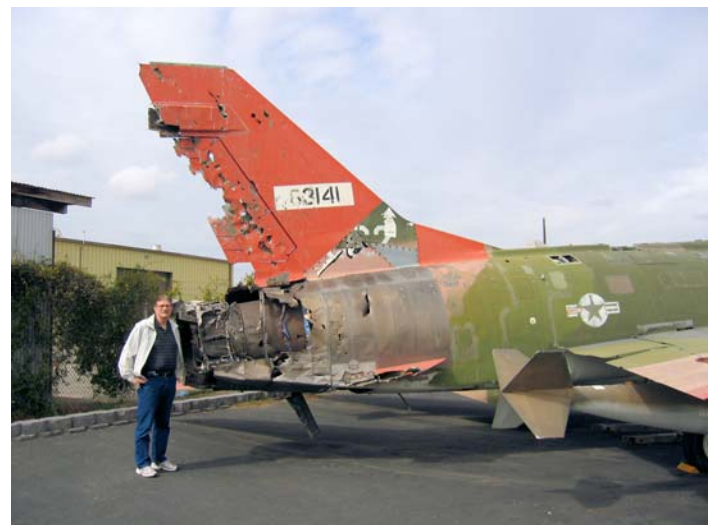
Ed O'Connor, checks out the damage to a QF-100 at the Chino, CA, air museum. This sturdy Hun survived an AIM-120 (AMRAAM) attack by an F-15!
