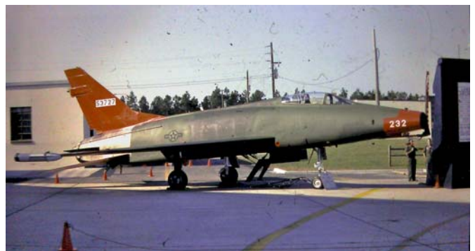
A QF-100D all spruced up for static display during a William Tell air-to-air gunnery meet at Tyndall. Drone mods you can see with a magnifying glass include the flare pod on the right wingtip to preserve the QF by decoying heat seekers. Also, along the aft fuselage is the Thunderbird smoke system; a long, thin tube which used engine oil sprayed into the exhaust plume to produce white smoke to mark the drone's position for the shooters. A number of small telemetry antennas are obvious in the nose area, along the dorsal line of the fuselage, and dotting the vertical tail.
