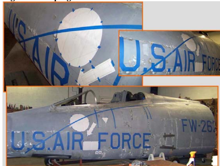
Figure 5 – Taping the Paint Job
