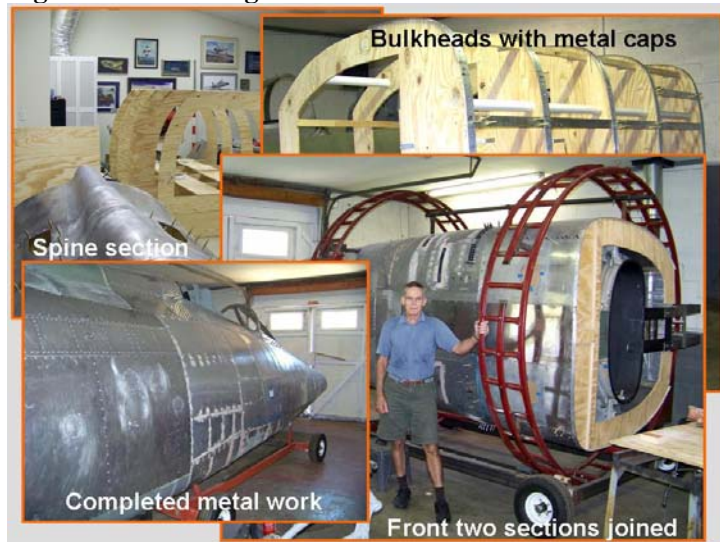
Figure 3 – Finishing the Metal Work
