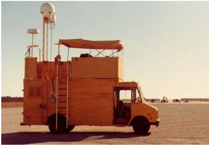
The MCU in takeoff position 800 feet behind the QF poised on the centerline. Takeoff was easy, but for landing, it was positioned off the runway, about 1,000 feet from the approach end. Given the parallax effect, that was where the Mobil Controllers really earned their pay. See Charlie Friend's anecdote below.
