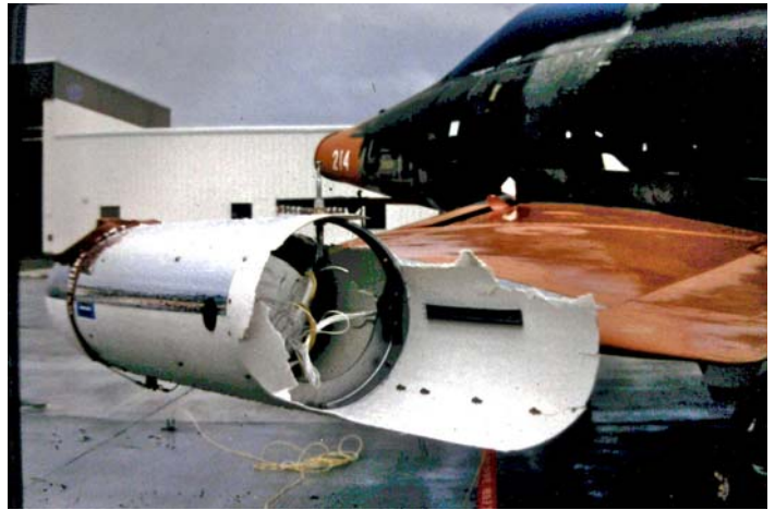
Yup. Here's a survivor with severe flare pod damage from an AIM-9
