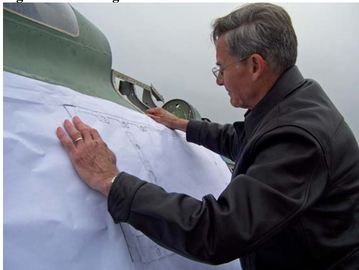
Figure 2 – Tracing Skin Plates
