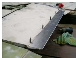
Aileron under repair.
