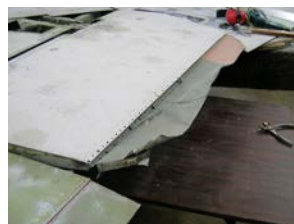
Damaged trailing edges.
