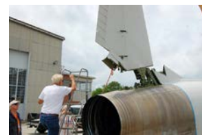
Vertical stabilizer goes on.
