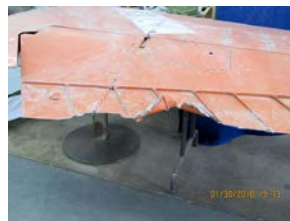
Damaged, corroded rudder.
