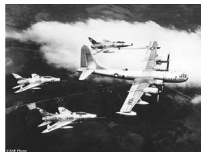
KB-50s could handle up to three aircraft at a time.
