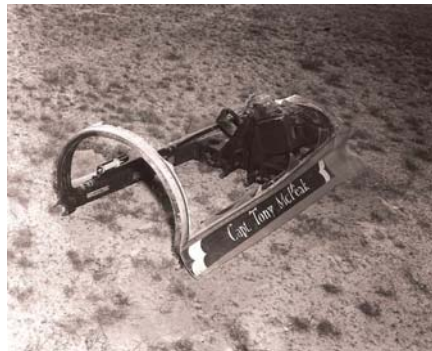
Unlike combat losses, Tony's canopy remains and all other debris were available for post-game analysis. Wing center box failure was identified as the culprit, and a fix was designed and implemented for the fleet.
