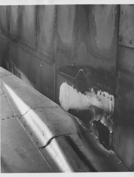
Engine fire damage.
